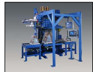
"A" and Flat Coil Heat Exchanger Assembly Test
