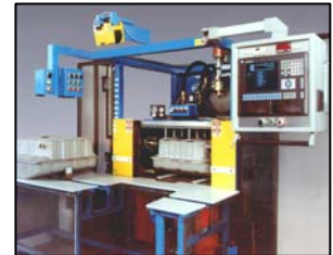
Fuel Tank Assembly Test
